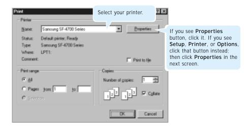
3. To take advantage of the printer features provided by the SF-4700, click **Properties** in the application's Print dialog box and go to step 4.
